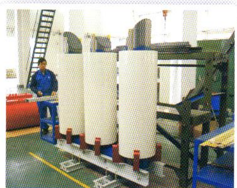
Core Coil Under Assembly
