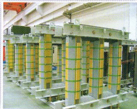
Transformer CRGO Core
